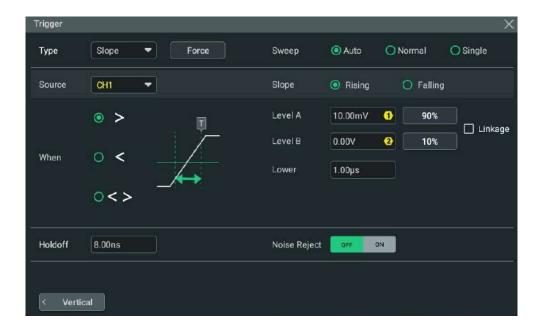
**Figure 8.7 Slope Trigger Setting Menu**
