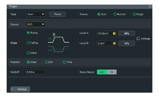
Figure 8.17 Window Trigger Setting Menu
