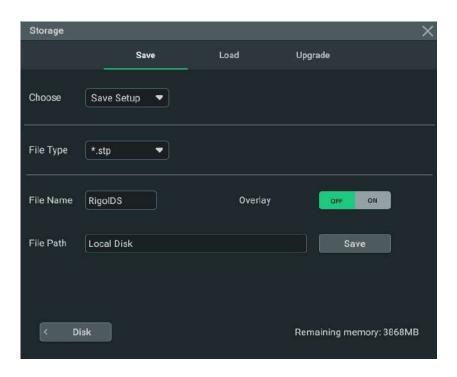
**Figure 20.3 Setup Saving Setting Menu**
