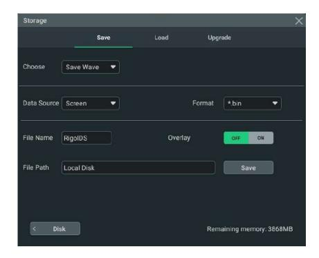
**Figure 20.2 Waveform Saving Setting Menu**
