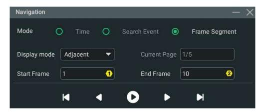
Figure 18.6 "Frame Segment" Navigation Setting Menu
