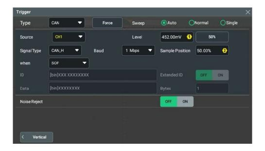
Figure 8.33 CAN Trigger Setting Menu
