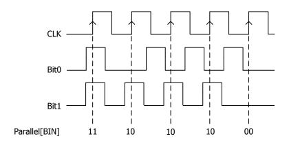
Figure 15.1 Schematic Diagram of Parallel Decoding
