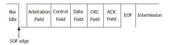
Figure 8.32 Data Frame Format of the CAN Bus
