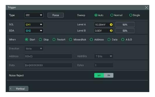
Figure 8.27 I2C Trigger Setting Menu
