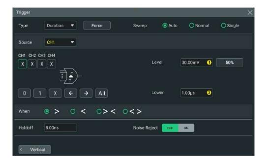
Figure 8.12 Duration Trigger Setting Menu
