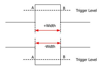
Figure 8.4 Positive/Negative Pulse Width
