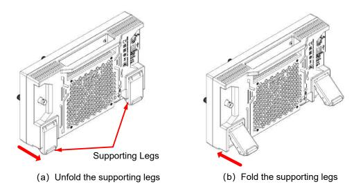
Figure 4.3 Adjusting the Supporting Legs
