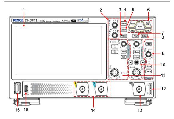
**Figure 4.9 Front Panel (2-channel Model)**
