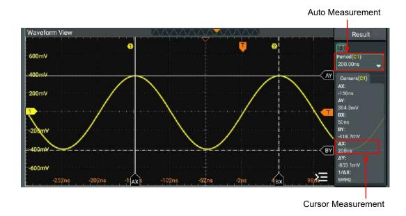
Figure 10.10 Manual Cursor Measurement Example
