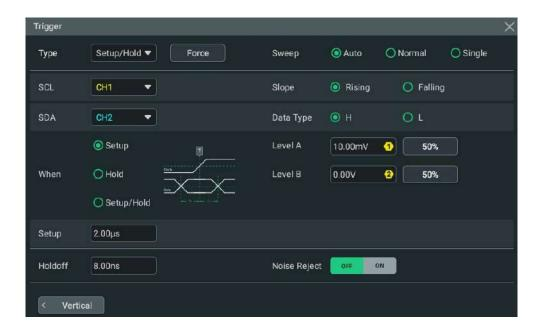
Figure 8.21 Setup/Hold Trigger Setting Menu
