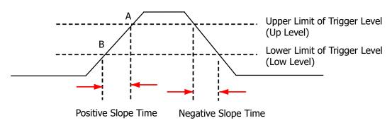
Figure 8.6 Positive Slope Time/Negative Slope Time
