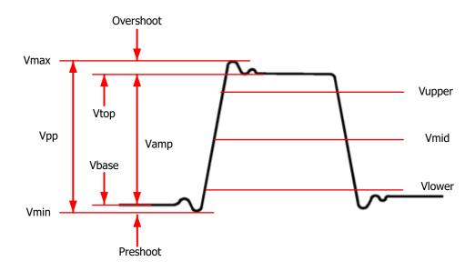
**Figure 10.3 Voltage Parameters**
