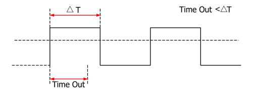
Figure 8.13 Timeout Trigger
