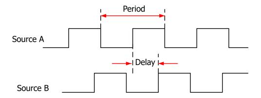
Figure 10.2 Delay and Phase Parameters
