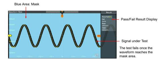
Figure 14.3 Pass/Fail Test Interface
