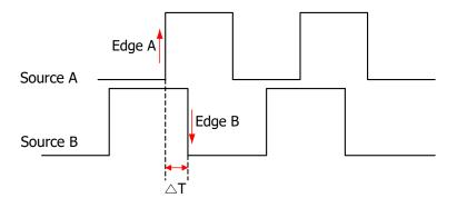
Figure 8.18 Delay Trigger
