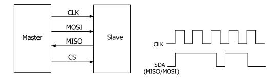
Figure 15.10 SPI Serial Bus
