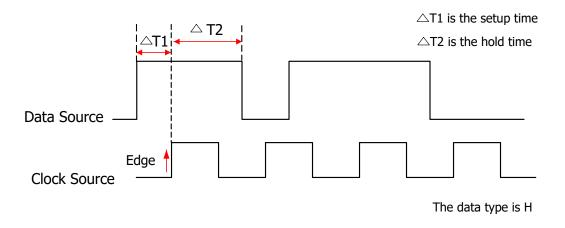
Figure 8.20 Setup/Hold Trigger
