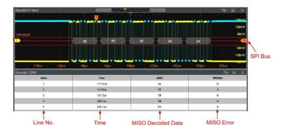
Figure 15.12 SPI Decoding Event Table
