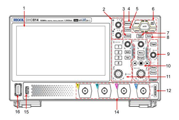
Figure 4.10 Front Panel (4-channel Model)
