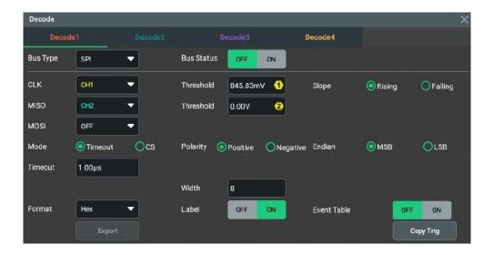
Figure 15.11 SPI Decoding Menu
