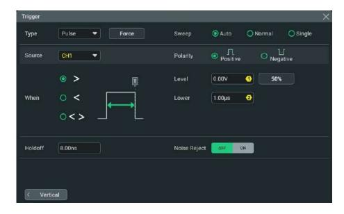
Figure 8.5 Pulse Width Trigger Setting Menu
