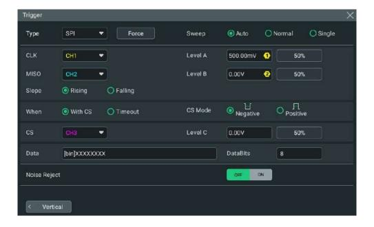
Figure 8.31 SPI Trigger Setting Menu
