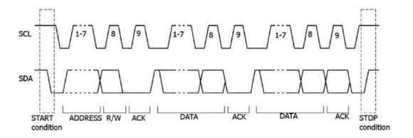
**Figure 8.26 Sequence Diagram of I2C Protocol**
