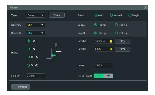
Figure 8.19 Delay Trigger Setting Menu
