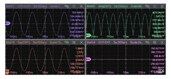
Figure 9.2 Waveform Display Window of the Operation Results
