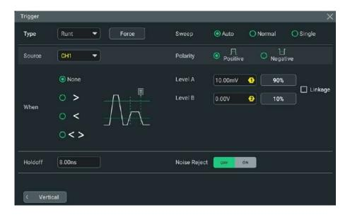
Figure 8.16 Runt Trigger Setting Menu
