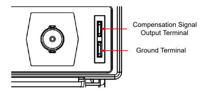
Figure 4.6 Using the Compensation Signal
