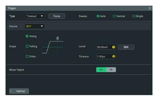
Figure 8.14 Timeout Trigger Menu
