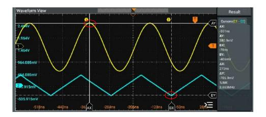
Figure 10.13 Track Measurement (after Horizontal Expansion)
