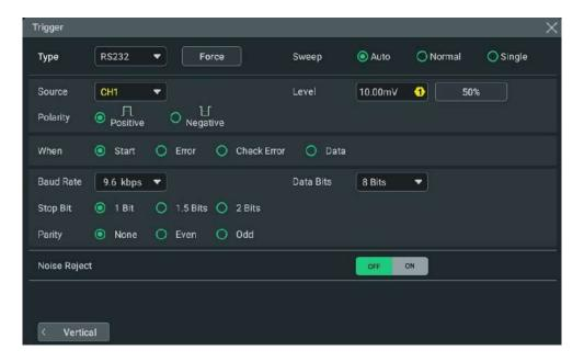
Figure 8.25 RS232 Trigger Setting Menu
