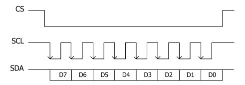
Figure 8.30 Sequential Chart of SPI Bus
