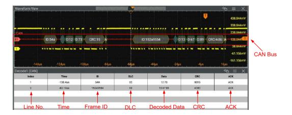
**Figure 15.15 CAN Decoding Event Table**
