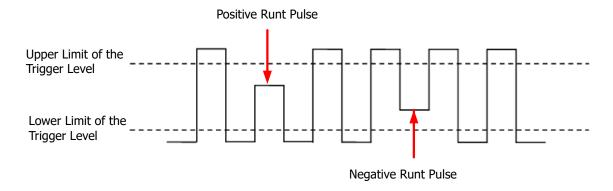
Figure 8.15 Runt Trigger
