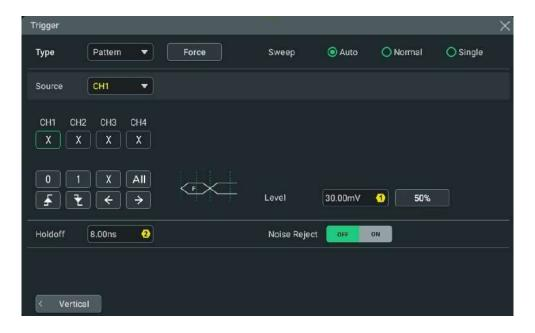
Figure 8.10 Pattern Trigger Setting Menu
