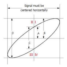
Figure 7.5 Measurement Schematic Diagram of Phase Deviation
