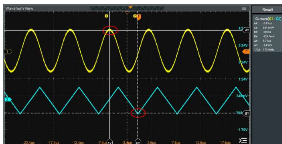
Figure 10.10 Track Measurement (before Horizontal Expansion)
