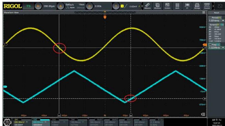
Figure 10.14 Track Measurement (after Horizontal Expansion)
