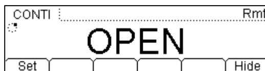
Figure 2-26 Continuity Testing Interface
