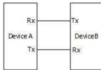
Figure 19.4 Schematic Diagram of RS232 Serial Bus
