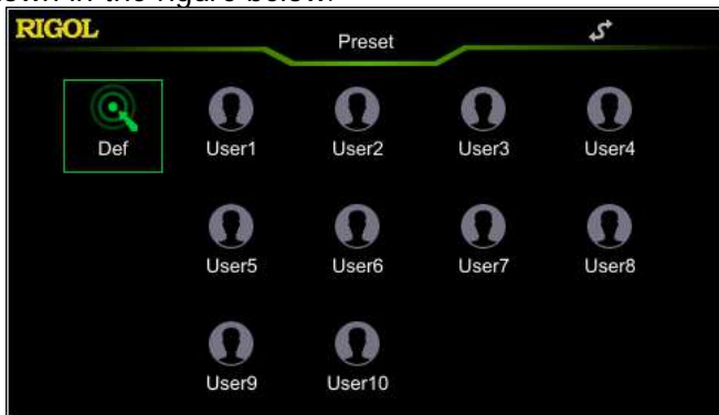
Figure 2-27 Preset Status Restore Interface
