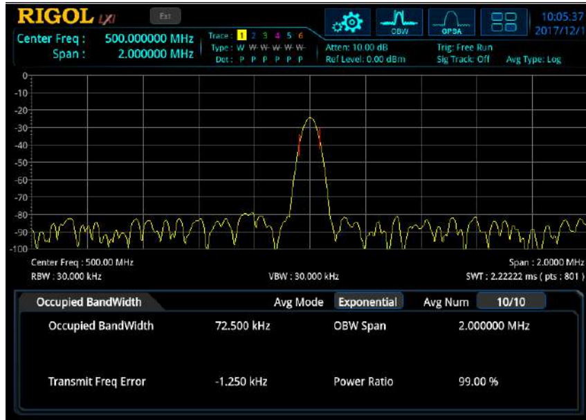
Figure 2-8 OBW Measurement Interface
