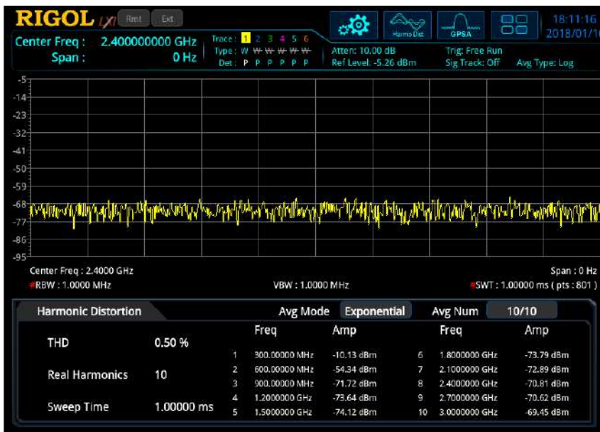
Figure 2-11 Harmonic Distortion Measurement Interface
