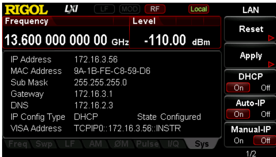
Figure 2-3 To Set the LAN Parameters
