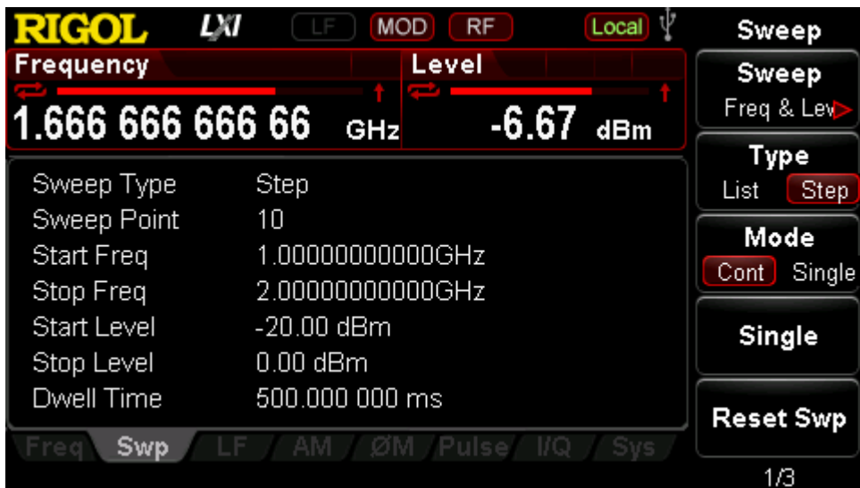
Figure 4-2 Parameter Setting Interface of RF Sweep Signal Output
