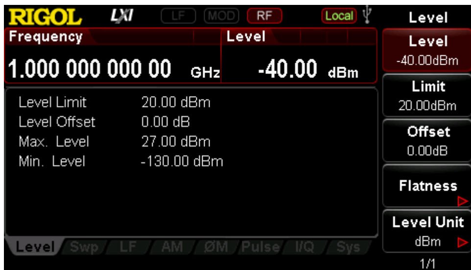
Figure 4-1 Parameter Setting Interface of RF Signal Output
