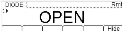
Figure 2-28 Testing interface of Diode
