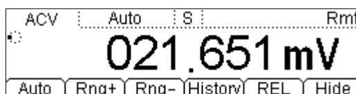
Figure 2-7 AC Voltage Measurement Interface
