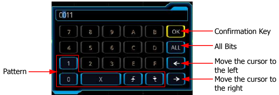
Figure 5-6 Virtual Keypad for Pattern Setting
