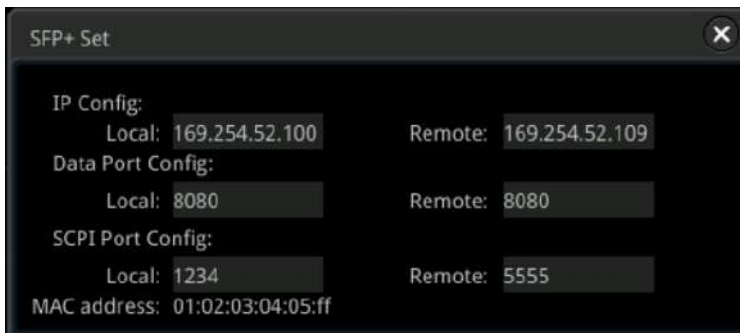
Figure 19-2 SFP+ Network Connection Setting Interface
