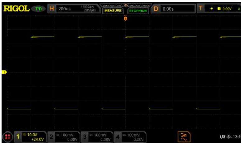
Figure 4-3 Waveforms after 128 Times of Averaging
