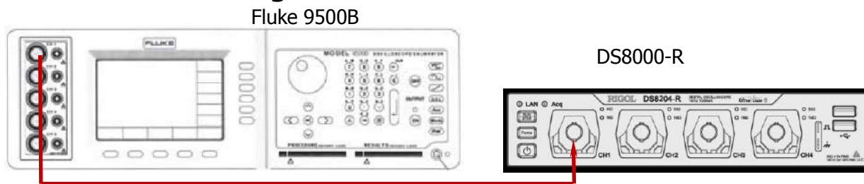
Figure 2-4 Bandwidth Limit Test Connection Diagram
