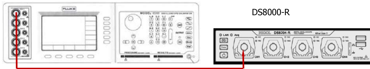
Figure 2-3 Bandwidth Test Connection Diagram
