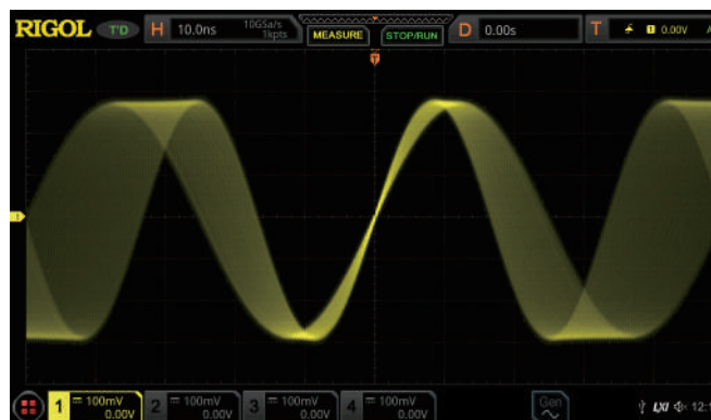
Changes of each frame of waveforms of the sweep signal can be clearly observed in the highly refreshed mode.
