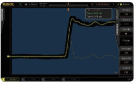
User-defined mask, Pass/Fail counts, stop on fail, fail alarm
