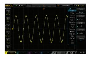
Built-in dual-channel 25 MHz source (DS1XX4Z-S Plus)
