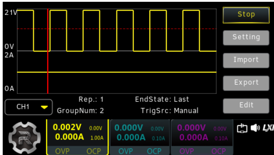
Figure 9.5 Arb Output Interface
